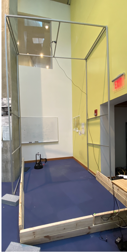
Figure 1: In this Figure, we can see the arena we built to collect the data and deploy the agent in the real world. It is bounded by wood studs, these were chosen as walls since it becomes easier to delimit the boundaries of the arena when using the point cloud camera (realsense2) on the LoCoBot. We additionally built a stand for another camera to have a third-person view of the entire arena.
